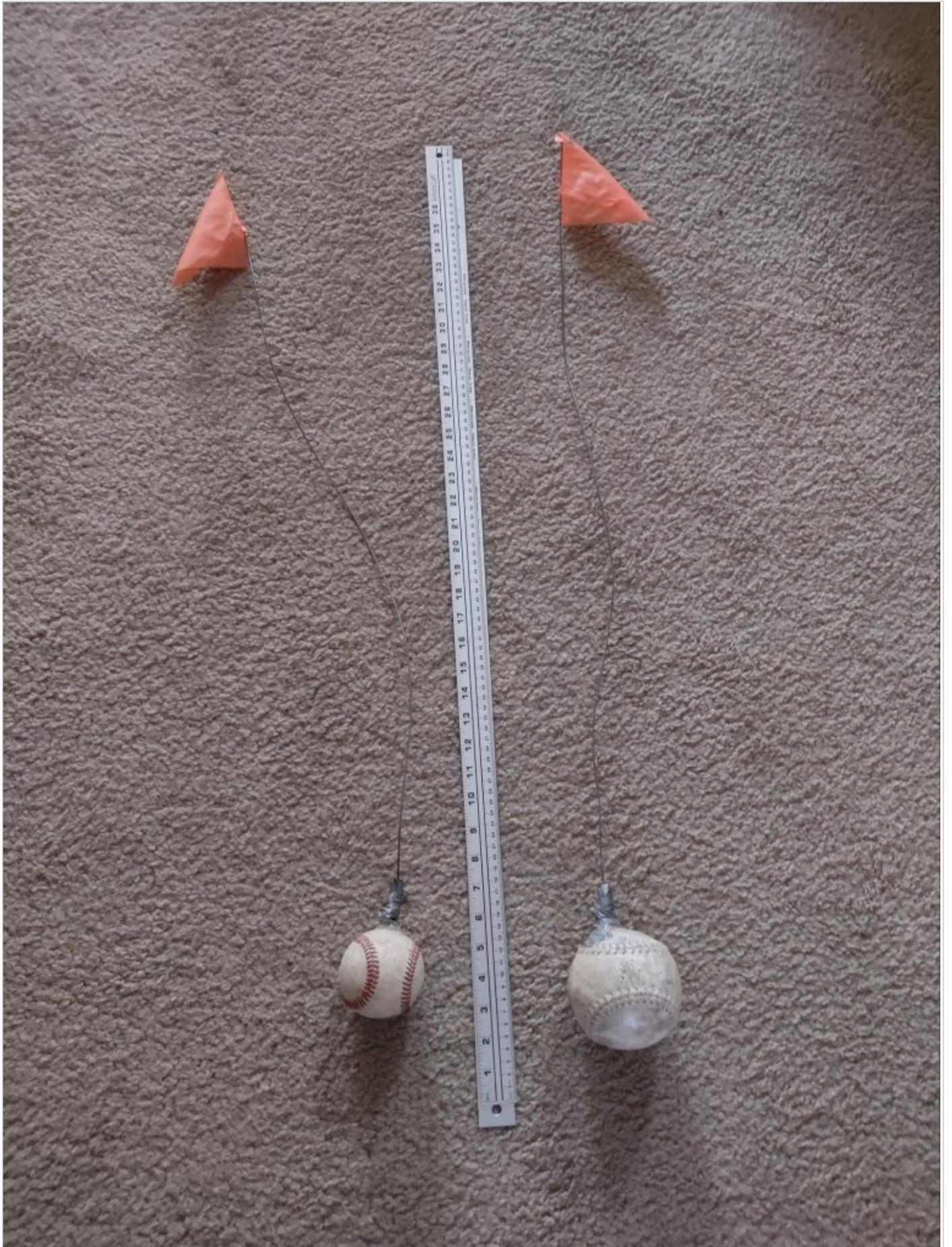
**Figure 1.** Baseball and softball tools used to measure depths in San Joaquin kit fox dens and California ground squirrel burrows on the campus of the California State University-Bakersfield, CA during June–July 2023.
