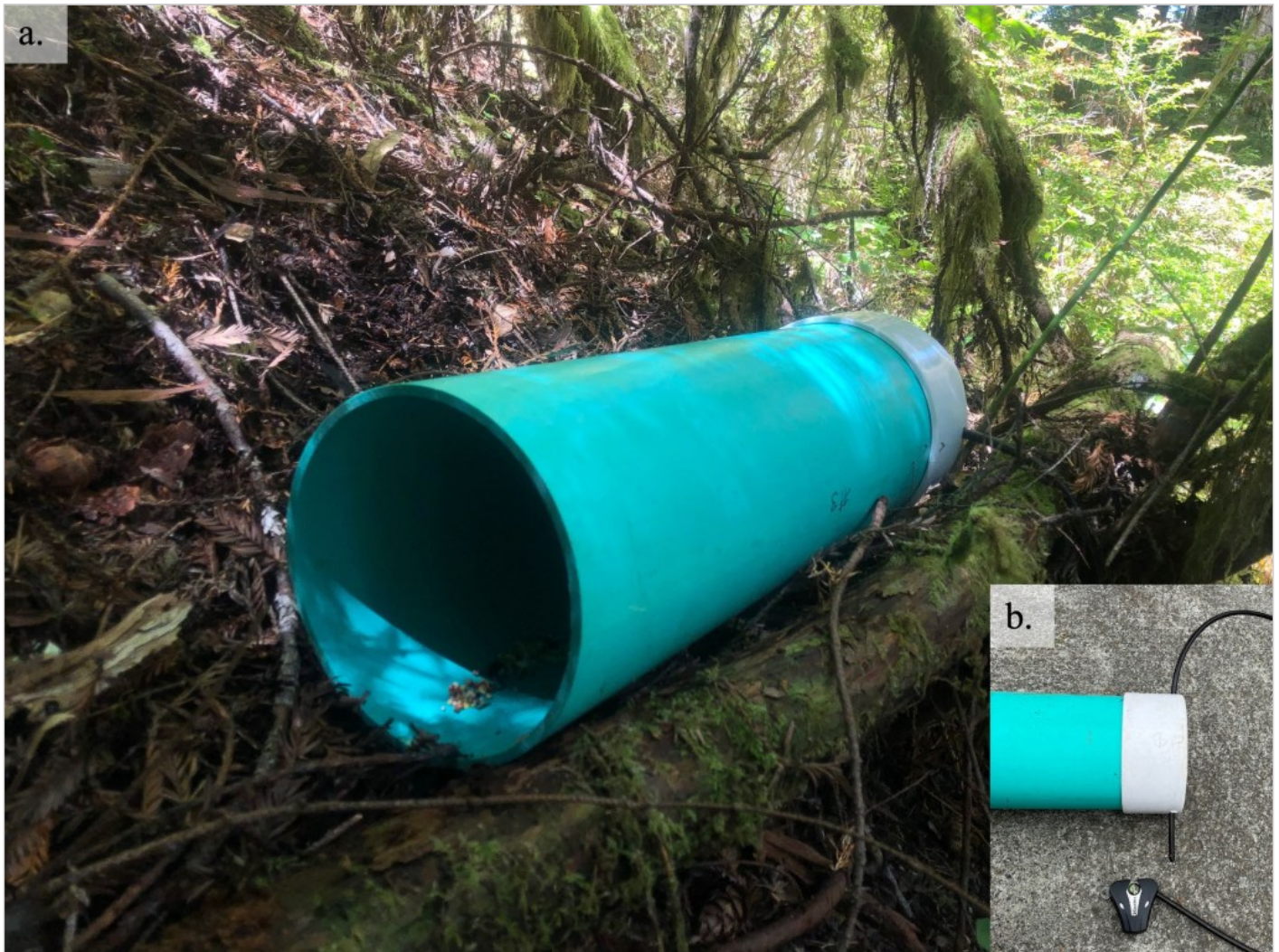
Figure 4. (a) Camera trap deployed in field, cable locked to downed log and tree, with bait (b) cable securing cap and camera on tube.
